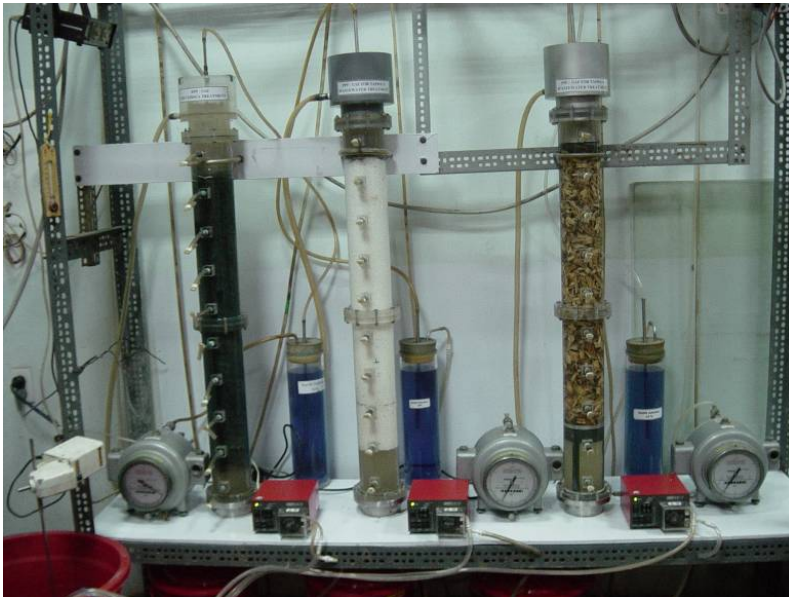
UASB-reactors and UAF-reactors (lab-scale) at the start-up period that are described in the thesis – CENTEMA laboratory
